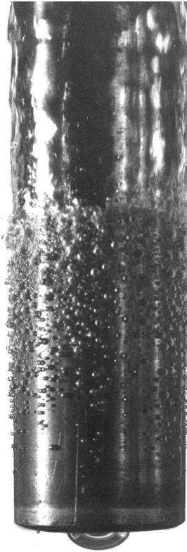
Figure 1: The evolution of convective boiling around a heated rod, reproduced from Sherman and Sabersky (1981).
