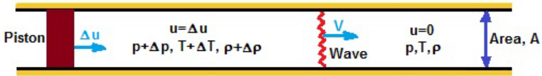
Figure 1: Tube with piston set in motion at t = 0 , with small velocity, \Delta u .
