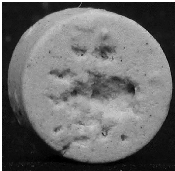
Figure 2: Artificial renal stone exhibiting damage (courtesy of Erin Hatt, Dept. of Anatomy and Cell Biology, Indiana University).
