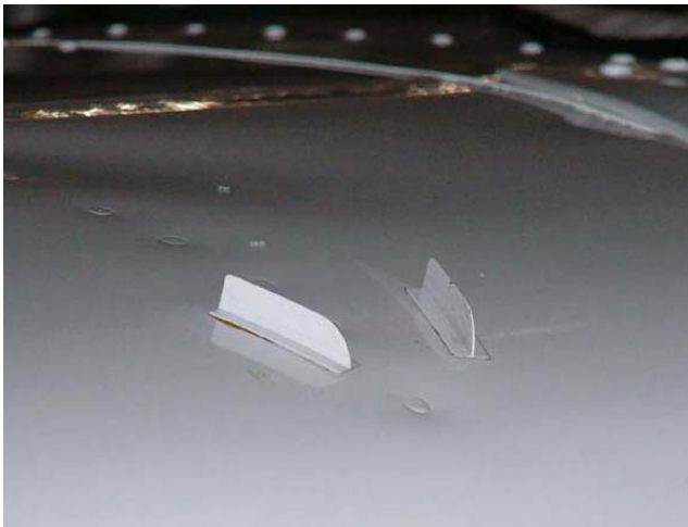
Figure 1: Left: Vortex generators on an aircraft wing. Right: Amy Williams, the 2010 Olympic Champion in Women’s Skeleton, with a helmet equipped with vortex generators.
