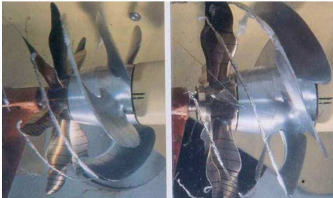
Figure 5: Tip vortex cavitation on counter-rotating propellers. Reproduced with permission of the Netherlands Maritime Research Institute and Lips B.V.
