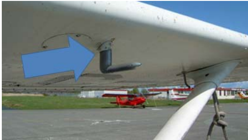
Figure 6: A Pitot tube mounted on an aircraft wing.
