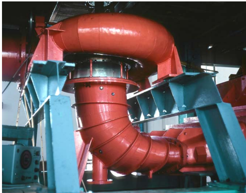
Figure 7: Turbine test facility at the Central Water and Power Research Station (CWPRS) near Pune, India, with a Francis turbine installed.
