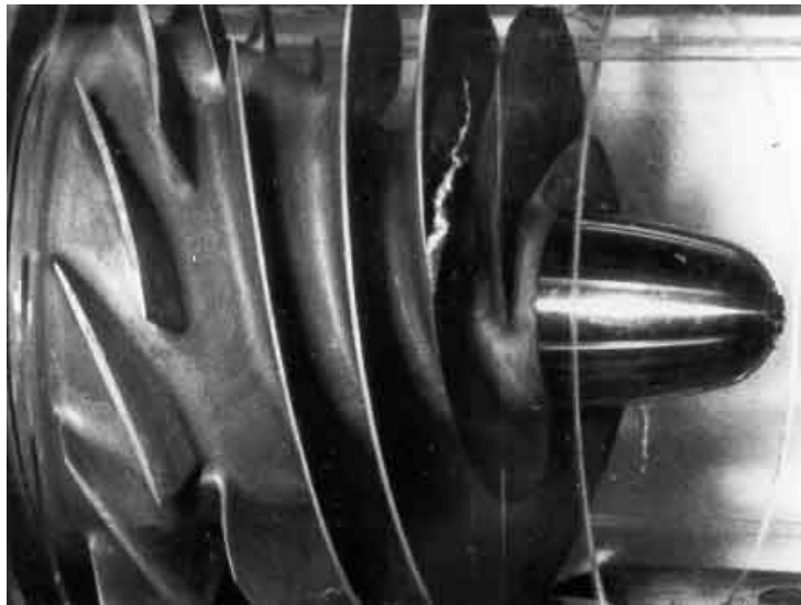
Figure 2: Cavitating tip vortex on a scale model of the low-pressure LOX turbopump impeller in the Space Shuttle Main Engine. The fluid is water, the inlet flow coefficient is 0.07 and the cavitation number is 0.42. Reproduced from Braisted (1979).
