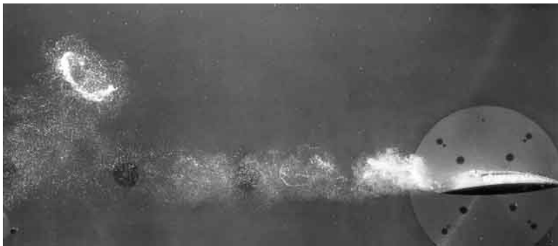
Figure 7: A vortex ring shed by the partial cavitation oscillations of a hydrofoil. The flow is from right to left. Reproduced with the permission of A.J. Acosta.
