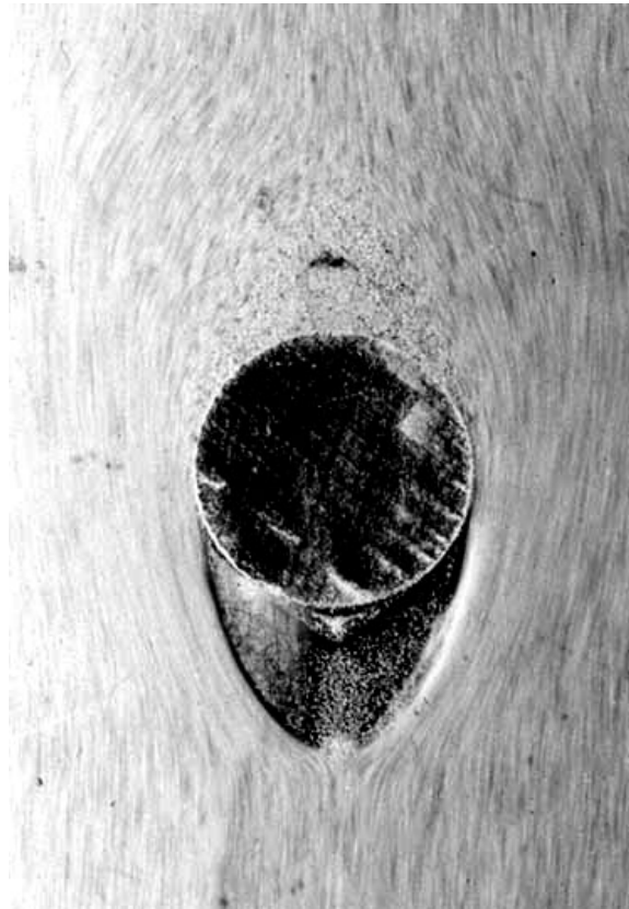
Figure 2: Long exposure photograph of the downward flow of sand around a circular cylinder. Reproduced with the permission of R.H.Sabersky.
