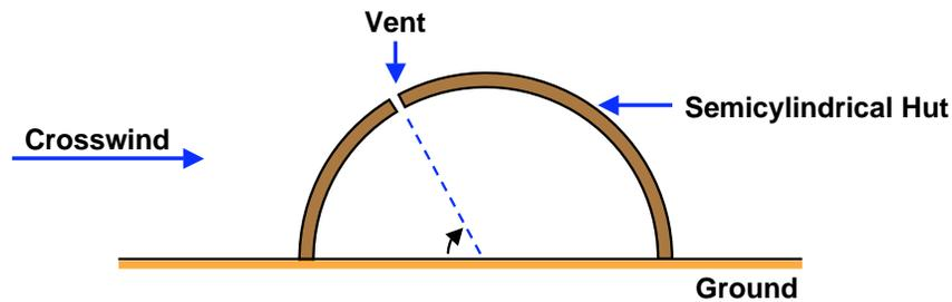
The interior of the hut is ventilated to the outside through a small vent at a position,  $\theta$ , as indicated. Hence the pressure inside the hut (assumed uniform and constant) is the same as the pressure just outside the vent. Assuming potential flow over the hut find the angle,  $\theta$ , at which the net vertical lift on the hut is zero. Neglect the thickness of the wall of the hut and assume that the vent has no effect on the exterior flow. Also assume that the air is incompressible.
