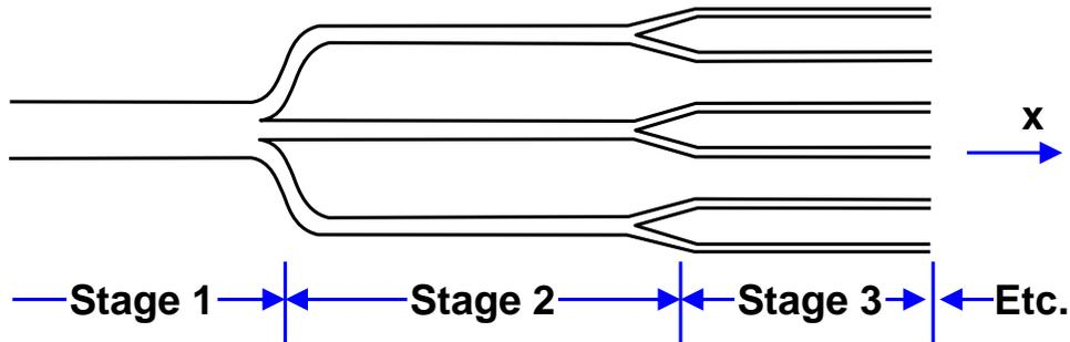
If, for each stage, the number of tubes is denoted by  $n$  and the cross-sectional area for each and every tube in that stage is denoted by  $A_n$ , find the relation between  $A_n$  and  $n$  such that the pressure gradient,  $dp/dx$ , is the same for each stage. How does the average velocity depend on  $n$ ? Assume steady, fully-developed Poiseuille flow in all tubes even though this may not be the case in the actual systems.
