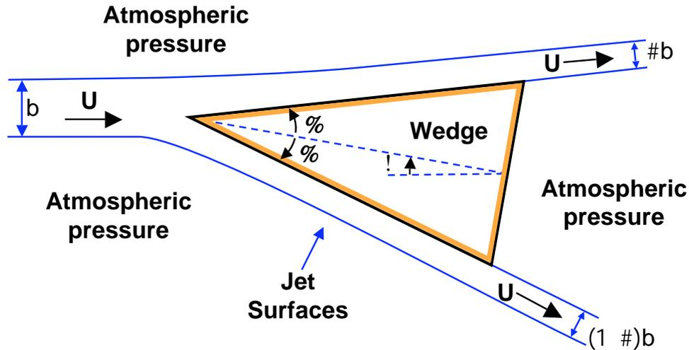
The angle of attack,  $\alpha$ , of the wedge is also defined in the sketch. The result is that the single incident jet is divided into two jets both of which leave the back edges of the wedge with the velocity,  $U$ . The widths of the two departing jets are  $\beta b$  and  $(1 - \beta)b$  as indicated in the figure. It is assumed that the flow is planar and that the pressure in surrounding air is everywhere atmospheric.
