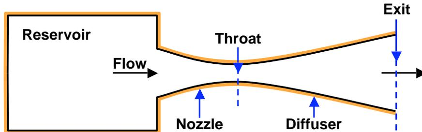
Assume the gas behaves like air ( $R = 280 \text{ m}^2/\text{s}^2 \text{ K}^\circ$ ,  $\gamma = 1.4$ ). The flow reaches critical conditions at the throat, is subsonic upstream of the throat and supersonic in the divergent section between the throat and the exit. The pressure at exit is atmospheric ( $10^5 \text{ kg/m s}^2$ ) and the supersonic flow at the exit is travelling at  $M = 2.5$ . Find:
