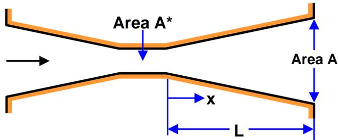
The nozzle is supplied from an air reservoir ( $\gamma = 1.4$ ) of pressure,  $p_0$ ; the external pressure of the air downstream of the diffuser exit is  $p_E$ . Find the ratio  $p_E/p_0$  at which a normal shock will form half-way along the diffuser, that is to say at  $x/L = 0.5$ .
