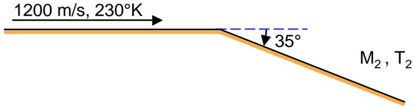
Find the Mach number,  $M_2$ , the temperature,  $T_2$ , and the velocity of the flow downstream of the corner. If the temperature of the upstream flow is lowered while its velocity remains at  $1200 \text{ m/s}$ , what is the theoretical minimum upstream temperature at which the flow will still be able to negotiate the turn?
