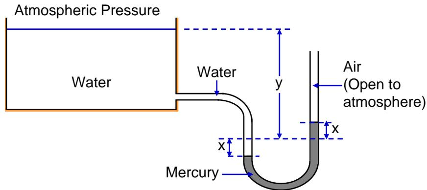
As the two fluids (water, mercury) are assumed to be incompressible, the hydrostatic relation can be used:
