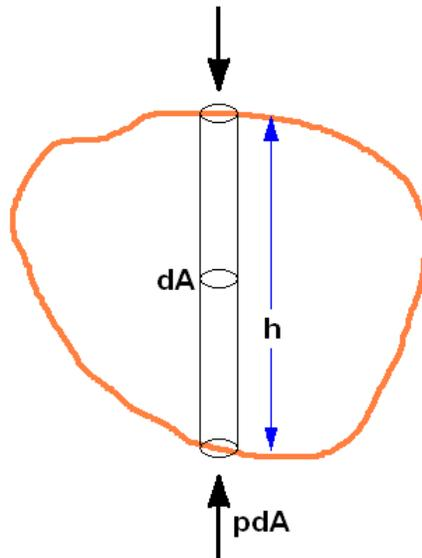
acting on a body immersed in a fluid as shown above. Consider a vertical cylindrical element of cross-section,  $dA$ , and length,  $h$ , and denote the pressure in the fluid at the lower end by  $p$ . Then the pressure at the top end will be
