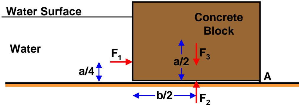
The forces on the rectangular block of concrete are:
