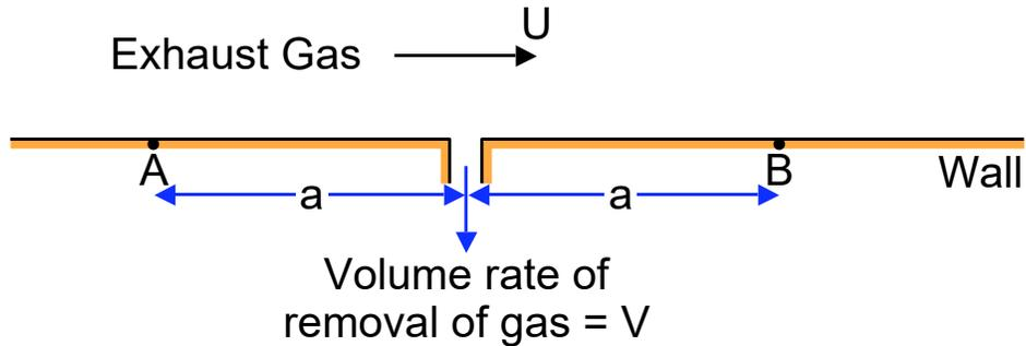
The volume rate of removal of gas,  $V$ , is simulated by placing a sink of strength  $2V$  at the location of the vent hole. Then the potential flow generated by the superposition of a uniform stream,  $U$ , and the sink of strength,  $2V$ , leads to a velocity,  $u$ , given by
