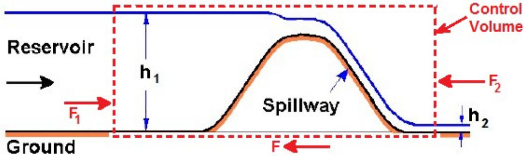
The depth downstream of the spillway is denoted by  $h_2$ . Consider the control volume indicated by the red dashed box in the above figure. Since the fluid is frictionless the forces acting on this control volume are the force  $F$  applied to the spillway to hold it in place and the pressure forces (per unit breadth) on the left,  $F_1$ , and on the right,  $F_2$ , where
