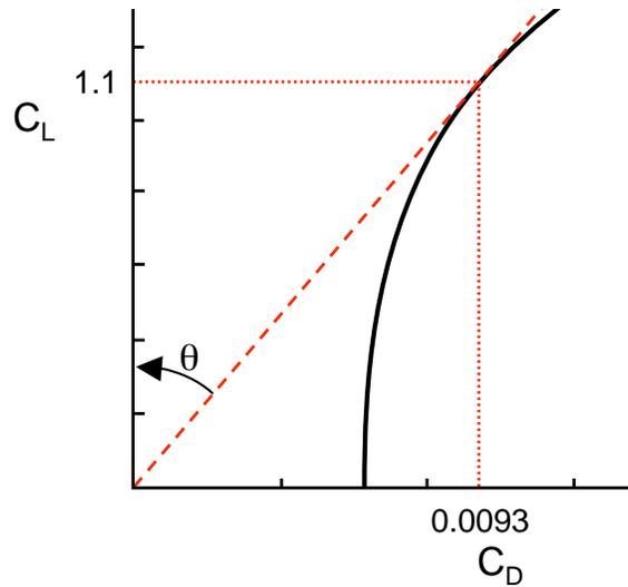
has a minimum met by the conditions at the point where  $C_L = 1.1$ ,  $C_D = 0.0093$ . Therefore the minimum glide angle is approximately  $0.48^\circ$ . [Note: If the fuselage drag was included, this angle would be much larger.] In gliding,
