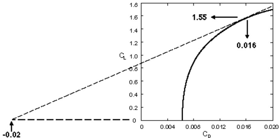
minimum glide angle,  $\beta$ , will be given by the values of  $C_L$  and  $C_D$  at the tangent point or
