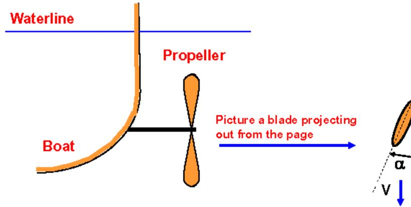
a velocity,  $V$ , and at an angle of attack,  $\alpha$ , so it produces lift in the direction of forward propulsion of the boat. The four blades therefore produce a thrust equal to
