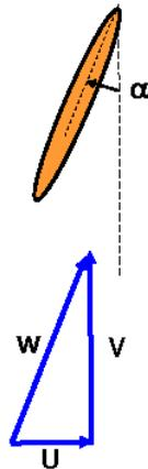
The angle of incidence with which the flow approaches the blade has now changed to  $\alpha - (U/V)$  (assuming small angles so that  $\tan^{-1}(U/V) \approx U/V$ ). Then the modified thrust is
