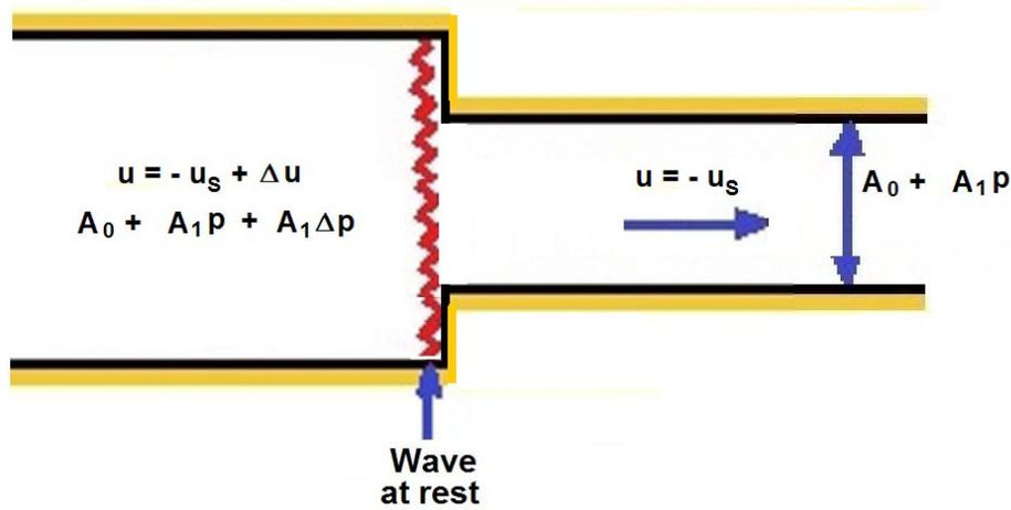
The conditions ahead of the wave in the undisturbed pipe the cross-sectional area:  $A = A_0 + A_1 p$ , the fluid velocity relative to the wave,  $u = -u_S$ , the fluid density is  $\rho$  and the pressure is  $p$  while the conditions behind the wave are:  $A = A_0 + A_1 p + A_1 \Delta p$ , the relative fluid velocity  $u = -u_S + \Delta u$ , the fluid density is  $\rho$  (since the fluid is incompressible) and the pressure is  $p = p + \Delta p$ .
