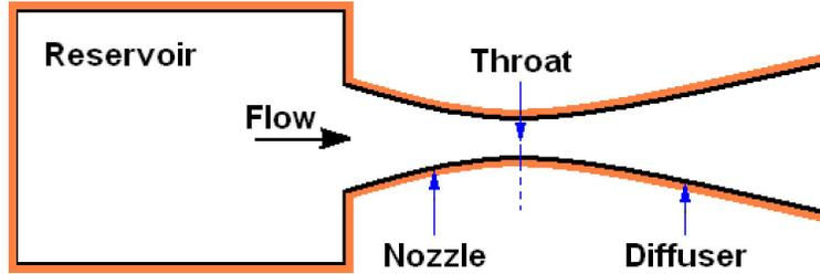
The flow reaches critical conditions at the throat, is subsonic upstream of the throat and supersonic in the divergent section between the throat and the exit. The pressure at exit is atmospheric ( $105\text{kg}/\text{ms}^2$ ) and the supersonic flow at the exit is traveling at  $M_{exit} = 2.5$ .
