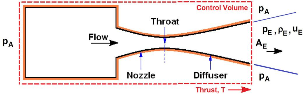
The flow reaches critical, choked conditions at the throat (Area  $A^*$ ), is subsonic upstream of the throat and supersonic in the divergent section between the throat and the exit. The pressure at exit (Area  $A_E$ ) is  $p_E$  and the surrounding atmospheric pressure is  $p_A$ . We wish to find an expression for the thrust produced by the engine in terms of  $p_0$ ,  $p_E$ ,  $p_A$ ,  $A^*$ ,  $A_E$  and  $\gamma$  (the ratio of specific heats).
