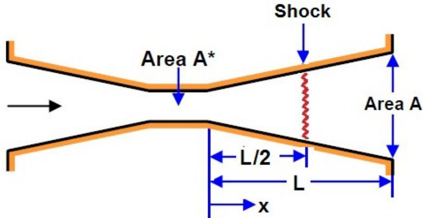
( $\gamma = 1.4$ ) of pressure,  $p_0$ ; the external pressure of the air downstream of the diffuser exit is  $p_E$ . We seek the ratio  $p_E/p_0$  at which a normal shock will form half-way along the diffuser, that is to say at  $x/L = 0.5$ .
