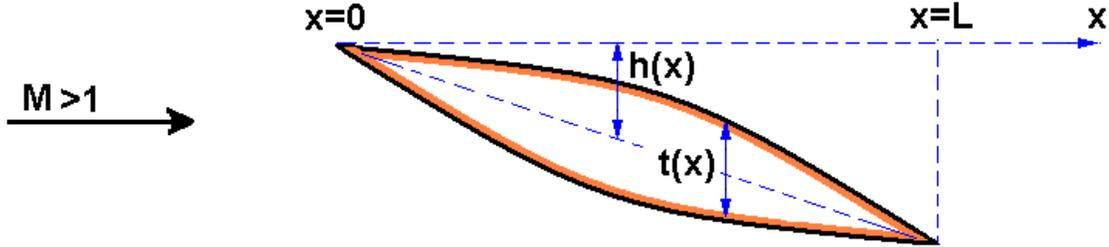
Denoting the pressure and velocity upstream of the foil by  $p_0$  and  $U$  then the pressures  $p_S$  and  $p_P$  on the suction and pressure surfaces are given by
