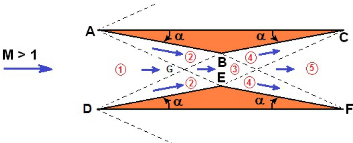
Downstream of the point G in region 3 the two flows must be turned so that they are parallel with one another. Therefore region 3 results from a second compression by the angle  $\alpha$  so that
