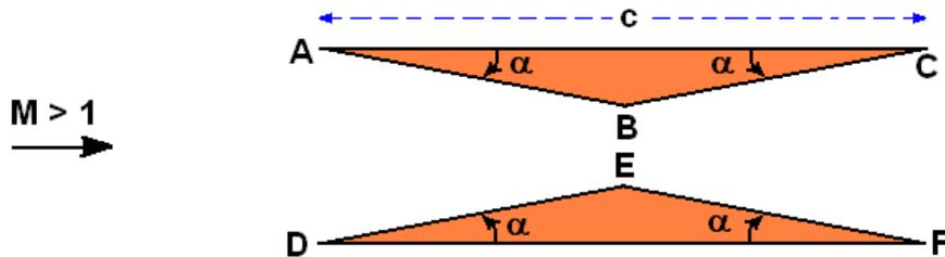
Since the angles  $\hat{BDF}$  and  $\hat{EAC}$  are both equal to the Mach angle,  $\mu = \arcsin(1/M)$ , Mach waves emanating from the points A and D will impinge directly on the vertices E and B respectively and since the flows in the regions 2 are compressed by the angle  $\alpha$  it follows that the pressures in the regions 2 will be
