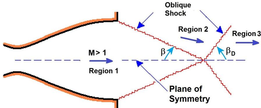
The flow exits the diffuser at a Mach number of 3.5. Because the surrounding atmospheric pressure is higher than the pressure of the exit jet, the engine is operating in an overexpanded mode and, hence, oblique shock waves occur emanating from the edges of the exit. These weak oblique shock waves are inclined at  $\beta = 25^\circ$  to the exhaust jet.
