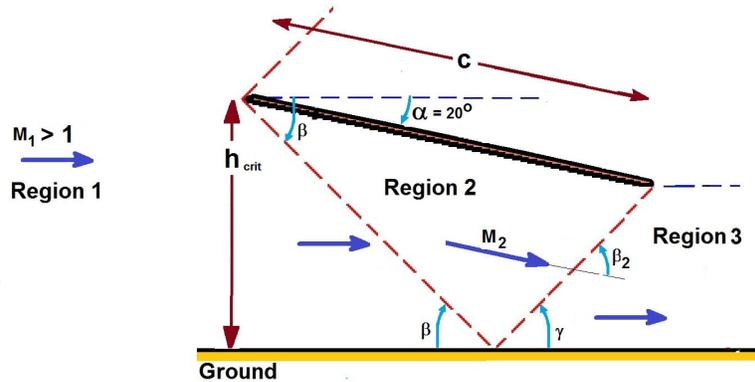
The oblique shock generated at the leading edge will be reflected by the ground and may or may not impinge on the foil. The critical clearance,  $h_{crit}$ , will be that at which the reflected shock just touches the trailing edge.
