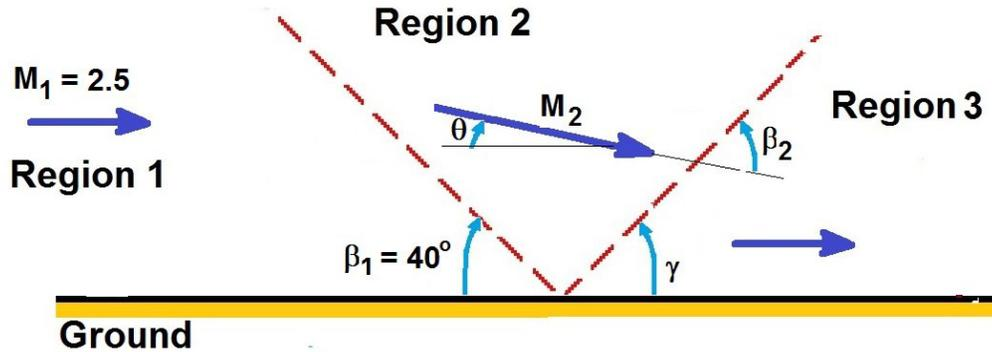
First analyze the incident shock wave whose upstream Mach number  $M_1 = 2.5$  and whose inclination to the incoming flow is  $\beta_1 = 40^\circ$ . From the oblique shock graph the flow deflection angle,  $\theta = 17.7^\circ$ . Also since  $M_1 \sin \beta_1 = 1.607$  from the shock wave table we find that  $M_2 \sin (\beta_1 - \theta) = 0.666$  and therefore  $M_2 = 1.755$ .
