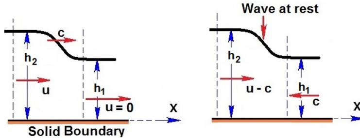
First we make a Galilean transformation from the frame of the question (the left-hand diagram) to a frame of reference in which the bore is fixed (the right-hand diagram). Then the analysis is identical with that of a stationary hydraulic jump and we can utilize the basic relation between the conditions on the two sides of the jump namely
